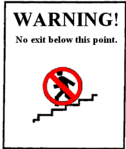
No. 2: Recommended sign inside Exit stairs below exit level.
