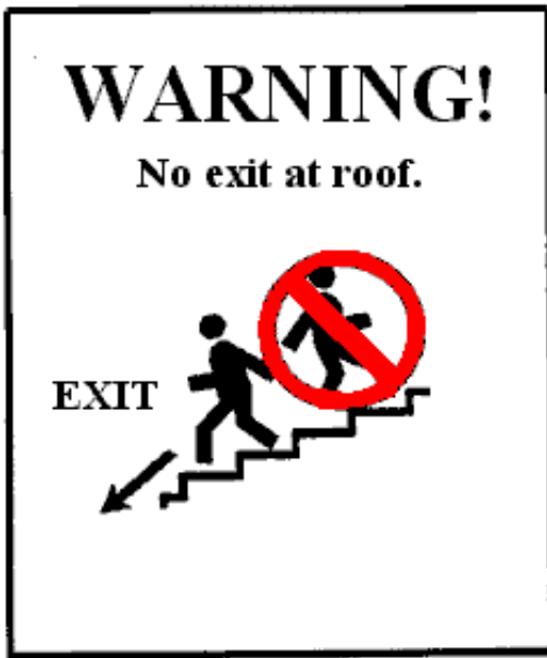
No. 1: Recommended sign to be Used throughout exit stairs
